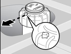
The watering area can be adjusted between 30° and 360°. When set to 360°, the nozzle does not reverse direction.
